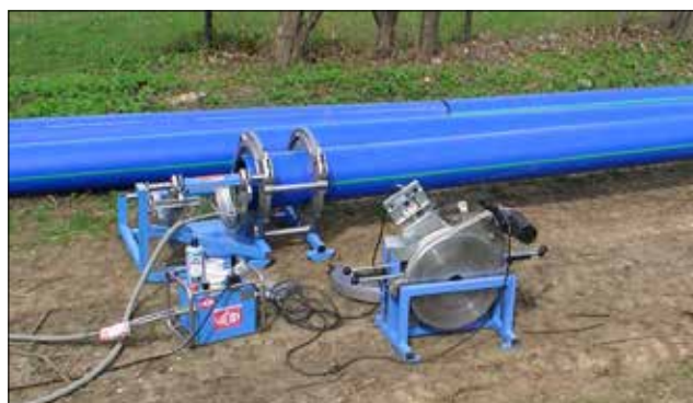
4.25 Gerodur service: provision of project-specific clamps for butt fusion (Widos) – delivery in robust heavy-duty box
