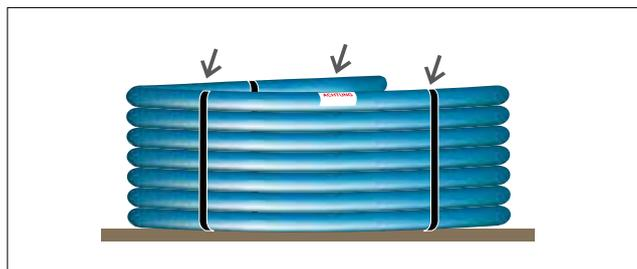
7.10 Correct storage of LHT® pipe coils
