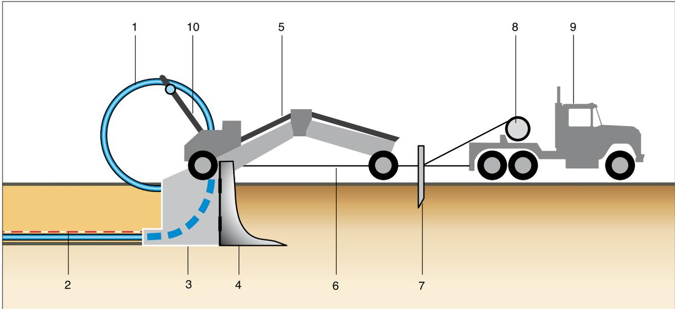
7.21 Ploughing | 1 LHT® piping | 2 utility marking tape | 3 laying box | 4 plough blade | 5 plough | 6 pulling cable | 7 support | 8 cable winch | 9 winch truck | 10 piping guide
