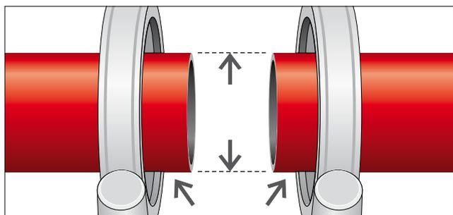
7.26 Clamp and align the pipes
