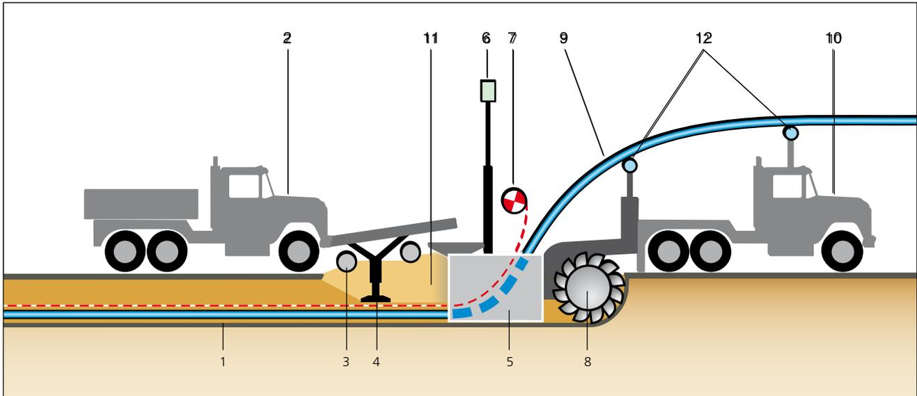
7.20 Narrow trenching | 1 trench bottom | 2 backfill and compaction unit | 3 axial screw conveyors | 4 compactor | 5 laying box | 6 laser receiver | 7 utility marking tape | 8 milling disc or cutter chain | 9 LHT® piping | 10 trenching and laying unit | 11 extracted material (spoil) | 12 piping guides
