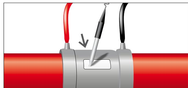
7.37 Scan the parameters (bar code), then weld and observe the cooling time
