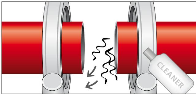
7.29 Remove chips and shavings in the jointing area and clean the fusion surfaces with PE cleaner
