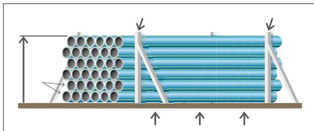
7.9 Correct storage of LHT® straight pipes without wooden framework
