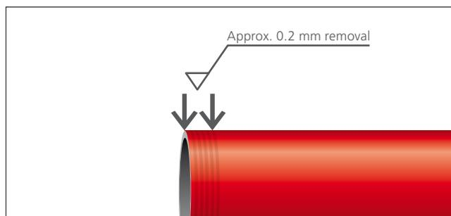
7.35 Machine the weld area, reliable with rotary peeler
