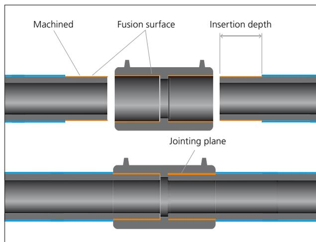
7.33 Principle of electrofusion welding
