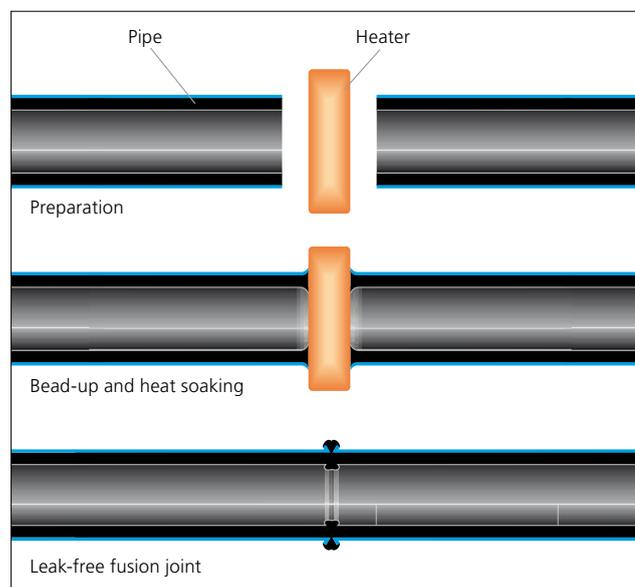
7.23 Principle of butt fusion welding
