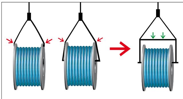
7.11 Loading and unloading of reels with a crane
