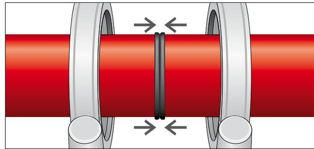
7.31 Changeover, jointing and final cooling under jointing pressure
